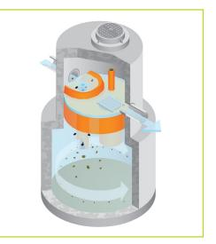
When the snow pile melts in the spring, the runoff flows down a specially-constructed asphalt pad to a series of catch basins and the Stormceptor. The Stormceptor slows the water and allows free oils to rise while sediment, with associated heavy metals and nutrients, settle and are held safely in the treatment chamber. The water then flows to a treatment pond for further treatment, and into a closed storm sewer system before discharging as clean water into a tributary of the Rouge River.
